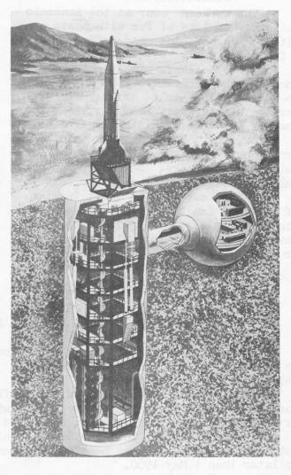
THESE CUTAWAY DRAWINGS show the prototype underground silo being constructed at Vandenburg AFB, Calif., for the Atlas ICBM to protect the missile against surprise enemy attack. At left, maintenance checkout and fueling operations are carried out underground in the silo containing the missile. At right, the Atlas has been raised and its rocket engines ignited. Countdown of the big missile is conducted in the spherical underground blockhouse at the right.
