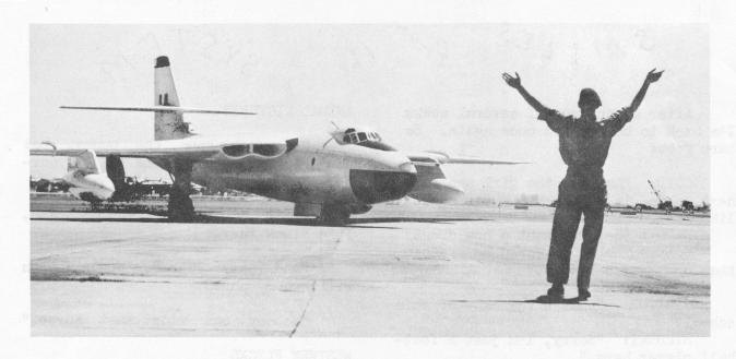
THE VICKERS VALIANT is a long-range, four-jet medium bomber in use by the Royal Air Force. Shown here at March AFB, California, the Valiant can be adapted to carry the Avro Blue Steel stand-off bomb with conventional or nuclear warhead. Its estimated max speed is 610 mph at 40,000 feet (Mach 0.925) and its service ceiling is 50,000 feet.
